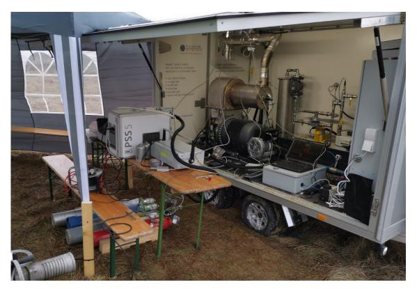
Figure 2: Measurement setup and Stirling cogeneration unit in the trailer.
