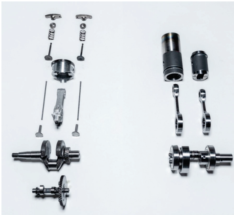
Figure 12: Ratio of the number of moving parts in a petrol engine (16) to those in a alpha-gamma Stirling engine (5)
