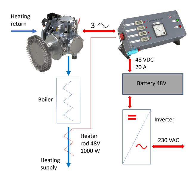
Figure 3: Simplified diagram of an experimental edition set for island power supply or grid connection. The heating rod is only required for charging control of the battery in stand-alone operation.
